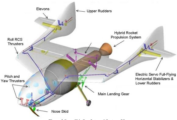
Figure 2 SpaceShipOne Internal Systems View
