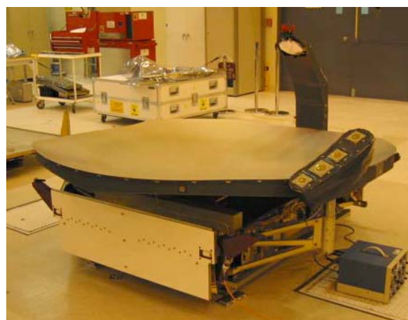
Figure 5: CPR Antenna Subsystem flight model.
