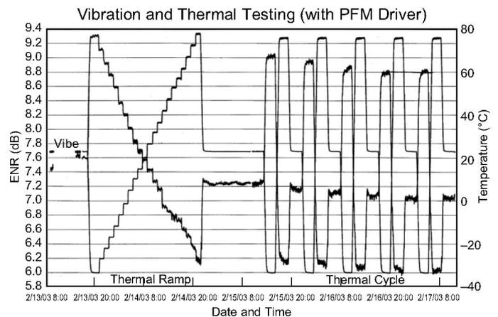
Fig. 9. Noise source burn-in test.
