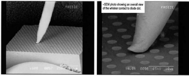
Fig. 6. Whisker contact – SEM photos: 600x and 4000x.
