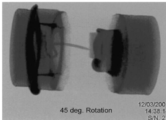
Fig. 5. Whisker diode – X-ray.
