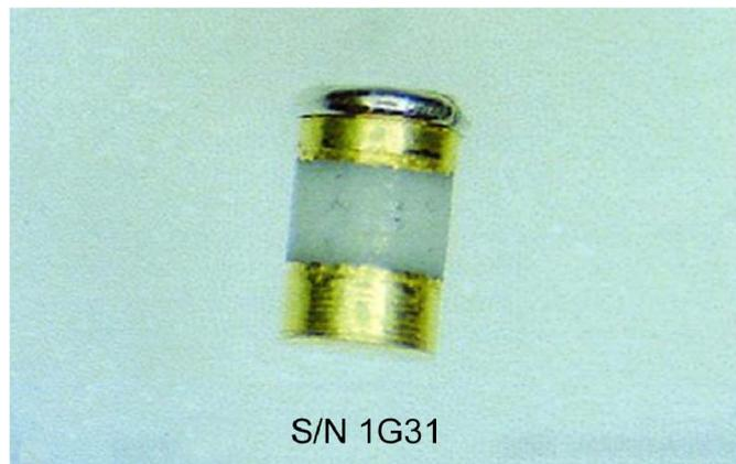
Fig. 4. Whisker contact diodes – hermetic package.
