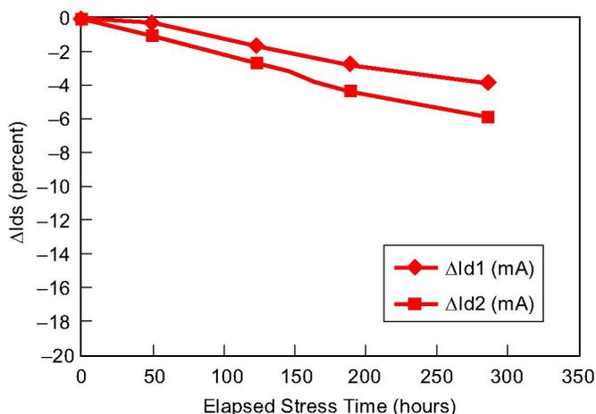
Fig. 11. MPA Ids vs. time for Pin = +17 dBm, T = 150°C.
