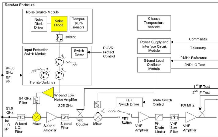
Fig. 2. Receiver block diagram.
