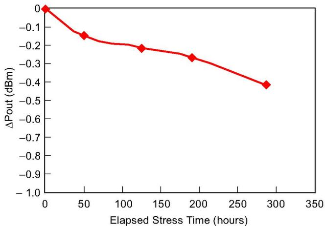
Fig. 10. MPA overdrive test – Pout vs. time for Pin = +17 dBm, T = 150°C.
