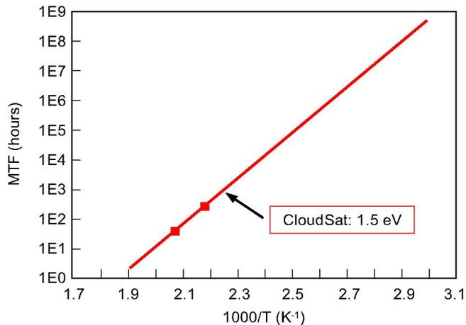
Fig. 13. LNA Arrhenius plot: 2-T lifetest, T = 175 and 200°C for activation energy = 1.5 eV.
