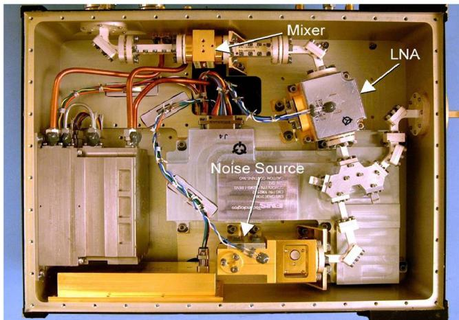
Fig. 3. Receiver W-band side.
