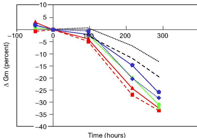
Fig. 12. LNA life test – Gm vs. time for T = 175°C for 8 samples.
