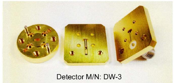
Fig. 8. W-band detector diode assembly.
