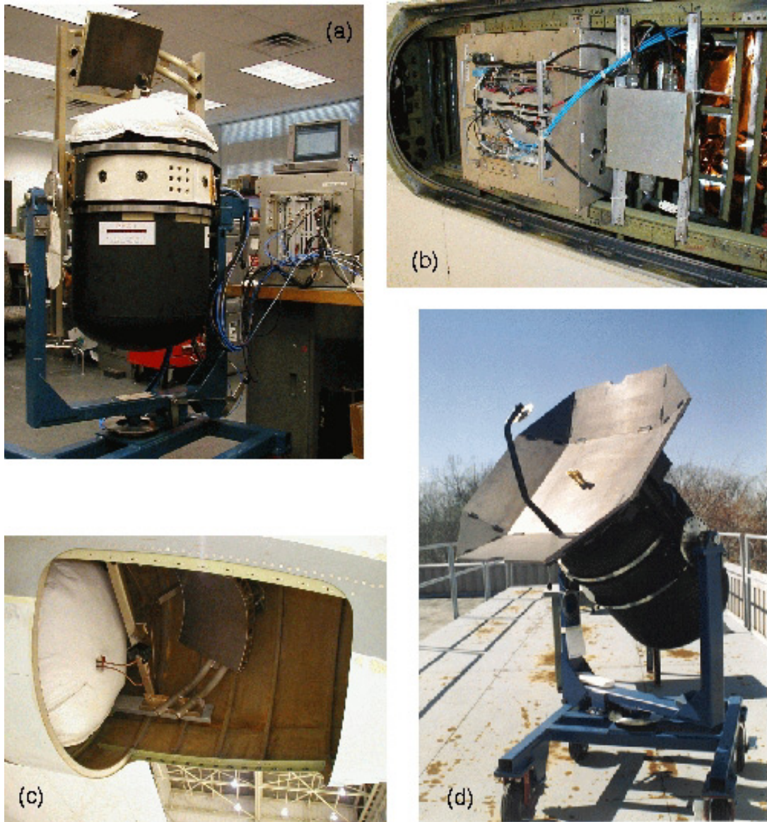
Figure 2. CRS hardware: (a) CRS setup in laboratory with the airborne antenna, (b) CRS data system installed in the middle body of ER-2 right wing pod, (c) CRS RF/IF subsystem installed in tail cone of ER-2 right wing pod, (d) CRS with the ground-based antenna mounted on the dual-axes gimbaled mobile cart.
