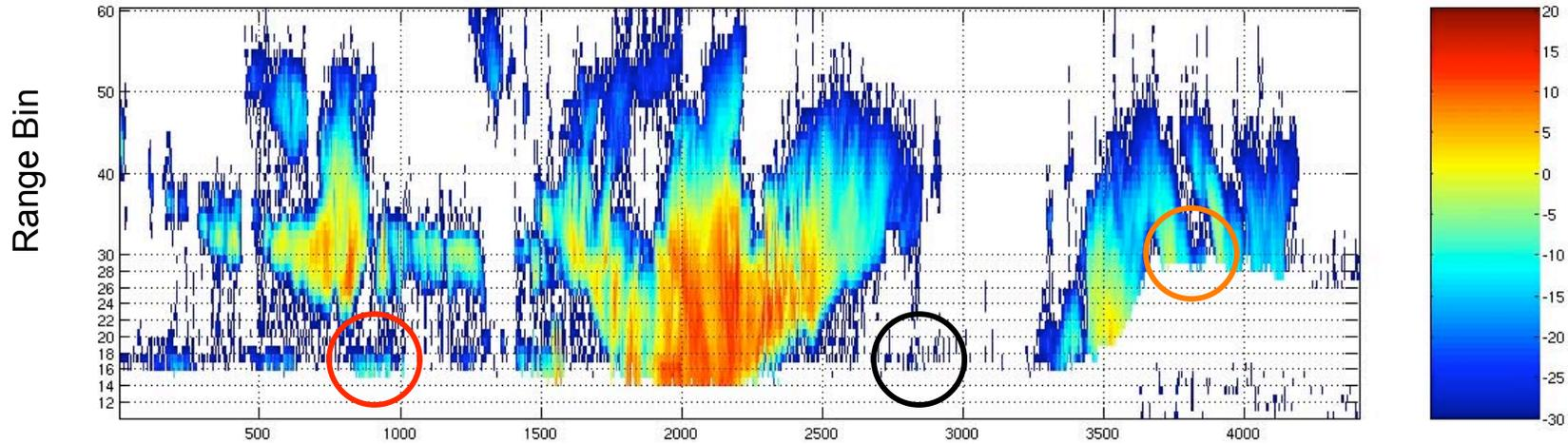
Z post-SCR with post\_SCR mask: 1-3 range bins above the surface are masked
