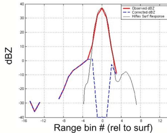
Z measured with CLDCLASS R03 mask: 3-4 range bins above the surface are masked
