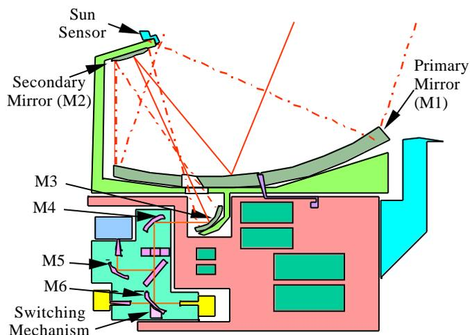
Figure 4. Graphical illustration of the CPR Antenna Subsystem.
