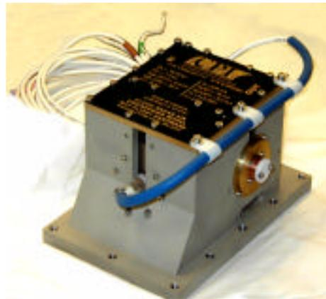
Figure 3. The second engineering model of the CPR's 94-GHz EIK.
