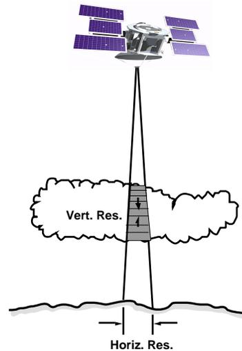
Figure 1. Cloud Profiling Radar (CPR) operational geometry.
