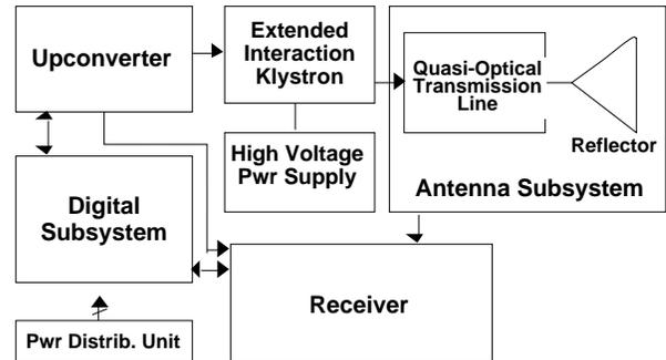
Figure 2. Simplified CPR block diagram.
