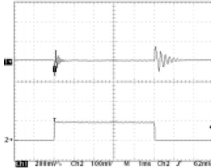
Fig 3—The transient response for 100 mA load step with  $C_{adj} = 0$  and  $R_{load} = 2.2 \text{ k}\Omega$  exhibits a 5-kHz ringing (upper trace,  $V_{out}$  200 mV/div; lower trace, load current 100 mA/div). Note that the ringing frequency is different on each edge of the step.
